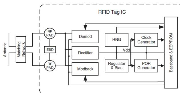
Gambar Blok diagram tag RFID
